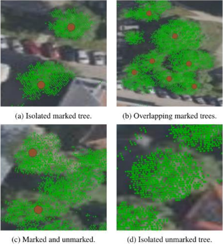
Figure 1: Panel (a) shows an ideal case for tree mining. Panels (b) to (d) depict point cloud and HD map mismatch issues.
